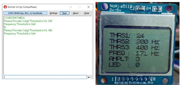
Before activating "A" and "B", each key is printed as it is. After "A" is pressed, the user is informed to input 3-digit, each digit is printed to the serial terminal. After 3-digit is entered, the corresponding threshold is updated in the Screen.
