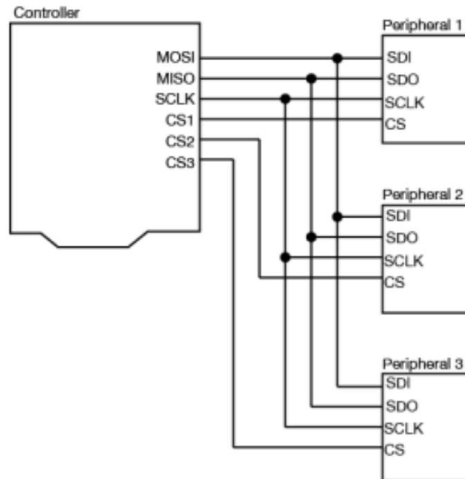
Figure 4: Synchronous Serial Interface in the TM4C
